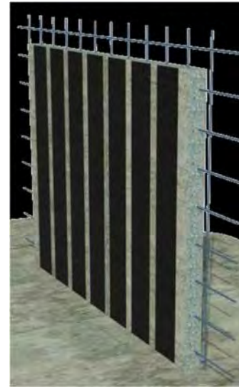
Wall Reinforcement (in/out-of-plane)
